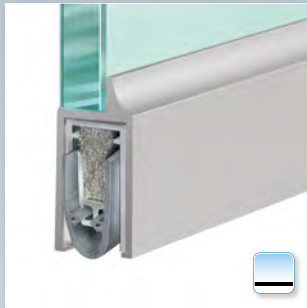
Planet KG-D8 | D10, UV-pasted from the bottom on glass door
